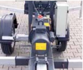
Push in axles, width clearance 0.89 m (optional)
