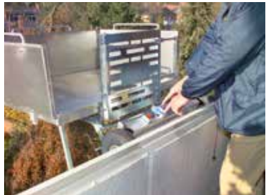
Operation from control unit at head piece*
