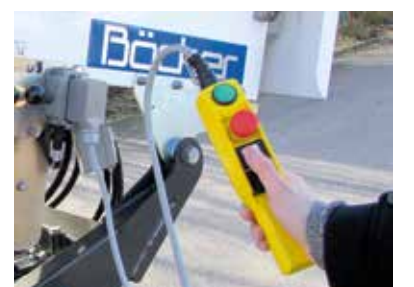
Operation below via operating buttons with 4 m cable
