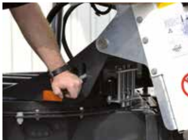
Adjustable turntable with mechanically releasable lock
