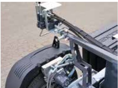
Powerful manoeuvring drive (optional)
