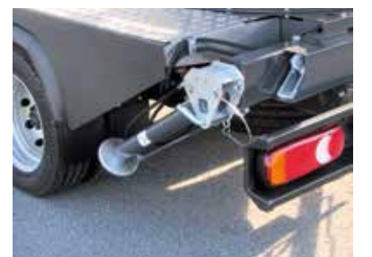
Hydraulic outriggers mechanically extendable and 60° swivelling
