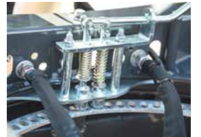
Infinitely adjustable turntable with mechanically releasable lock
