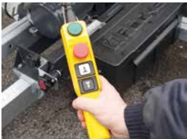
Electronic control with creep speed (optional)
