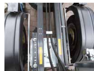
Retractable axle, manoeuvring width 0.89 m (optional)
