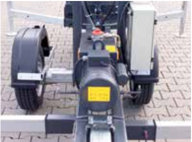
Retractable axles for manoeuvring width of 0.89 m (optional)
