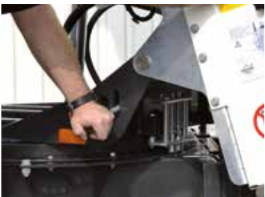
Adjustable turntable with mechanical lock release mechanism
