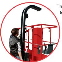
The setup of this device requires no tools and it is very fast. Once the job is completed, it is quickly removable for easy storage.
