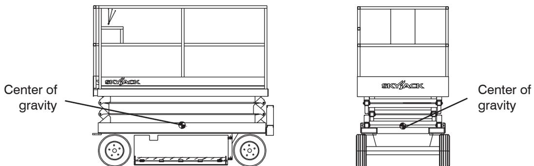
Figure 3-15. Center of Gravity
