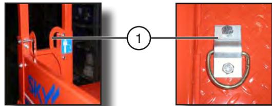
Figure 3-7. Lanyard Attachment Anchorage
