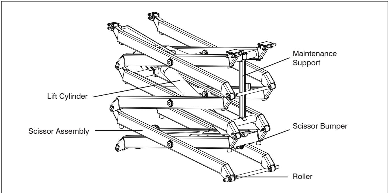
**2.3-9 Lifting Mechanism**
