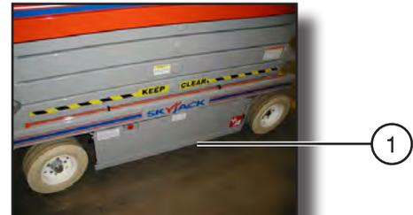
Figure 3-4. Pothole Protection Device
