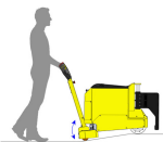
Self-adjusting castor guard for foot protection
