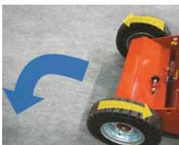
Allows the GL351® to turn "on the spot". The turning radius is not more than its own length, because the differential adjust the rotation of the front wheels automatically.
