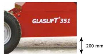
Ground clearing height of 20 cm combined with rugged tires give semi-off-road capabilities and building site access. The powerful drive allows the machine to drive uphill as well as downhill fully loaded.
