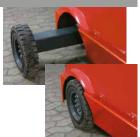
The front wheels are mounted on sturdy, stable, square axles that can slide to the sides. This gives the GlasLift® 500 unique stability.
